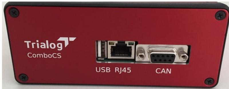
Figure 1: ComboCS connectors - Face 1
