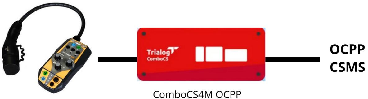
Or a CCS EV simulator like the EV ComboCS4M:
