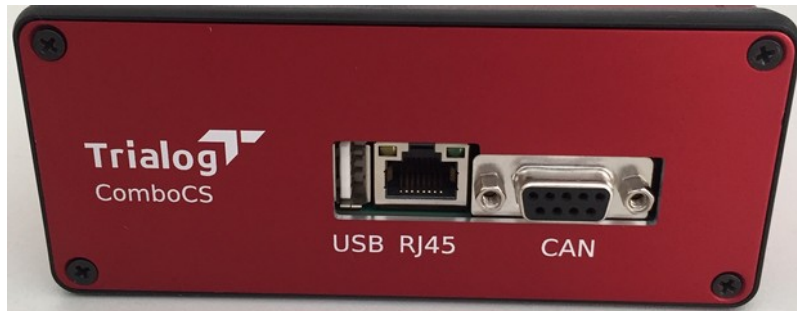
Figure 1: ComboCS connectors - Face 1
