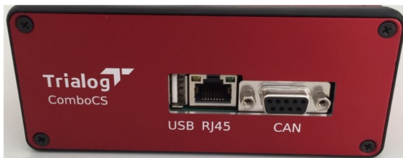
Figure 2: ComboCS connectors - Face 1
