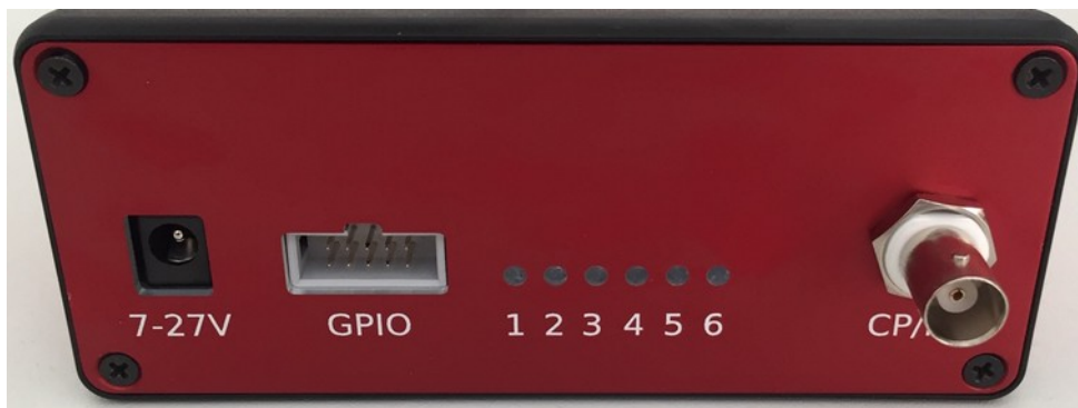
Figure 3: ComboCS4M showing session progress with LEDs
