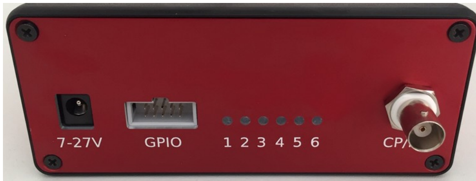
Figure 2: ComboCS4M showing session progress with LEDs
